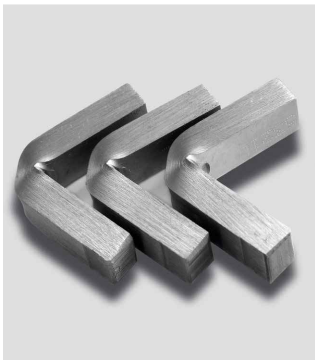
Impact bending samples (tempered to 44 - 46 HRC) after testing on a 450J pendulum impact testing machine
