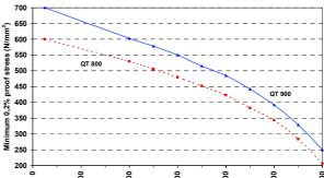
The temperature-stress-time relationships that are important for 1.4923 from a creep point of view are presented in the graph below:
