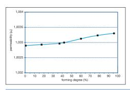
The diagram shows the variation of permeability against cold forming degree.
