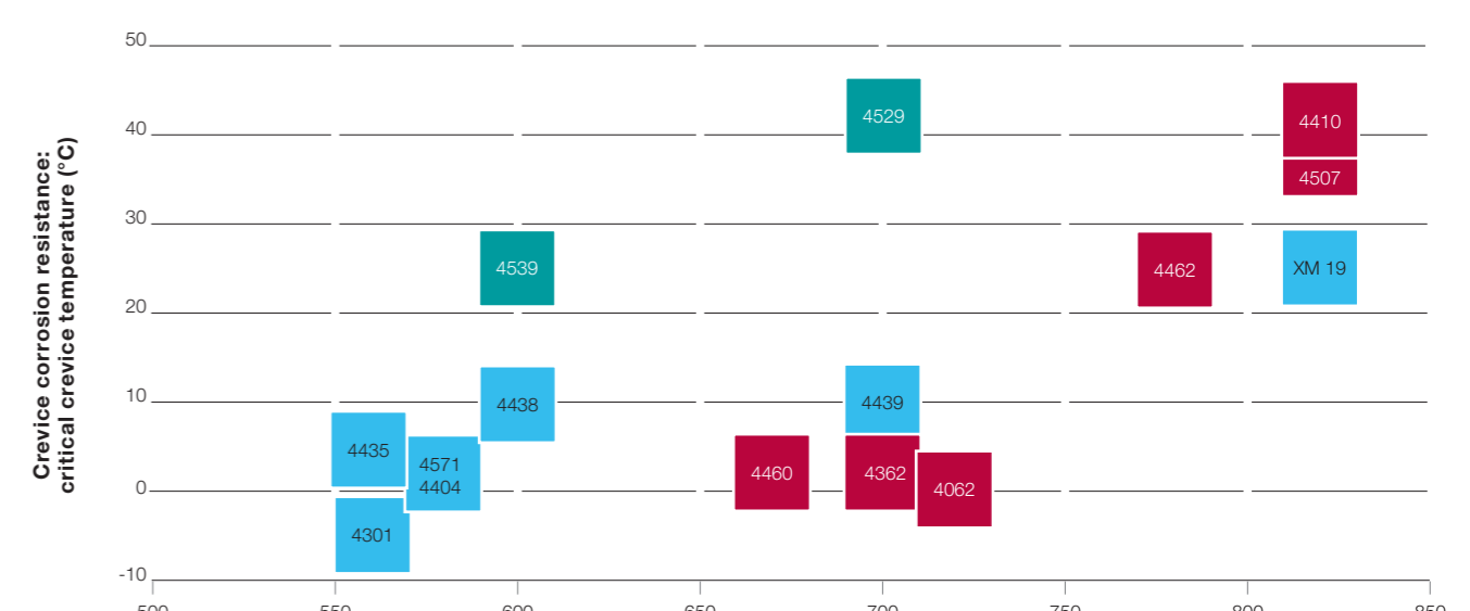
Mechanical properties: Rm (MPa) Crevice corrosion - Type testing using ASTM G48 in ferric chloride solution – indicative values
