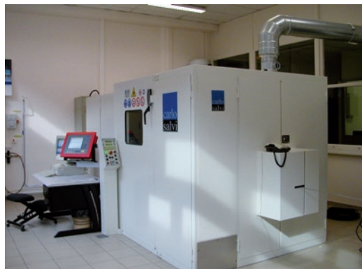
Industrial cold heading machine with instrumentation to assess the performance of our products
