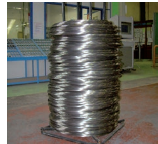
Spider - Weight = 800kg max - Int. Ø = 450 or 510mm - Base Ø = 850mm - Height = 1m or 1.30m
