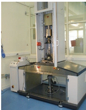
Drop weight device to determine the stainless steel behaviour law depending on strain rate and temperature (20 to 300°C)
